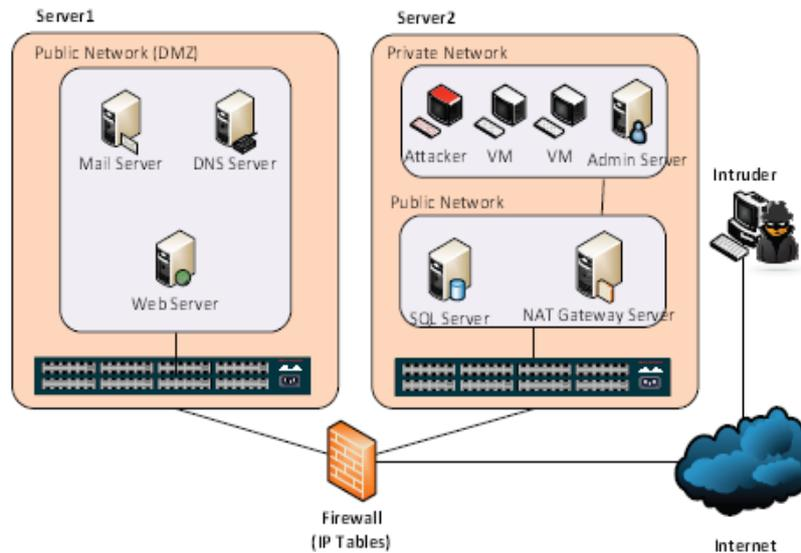
Fig.2: Virtual network topology for security evaluation
