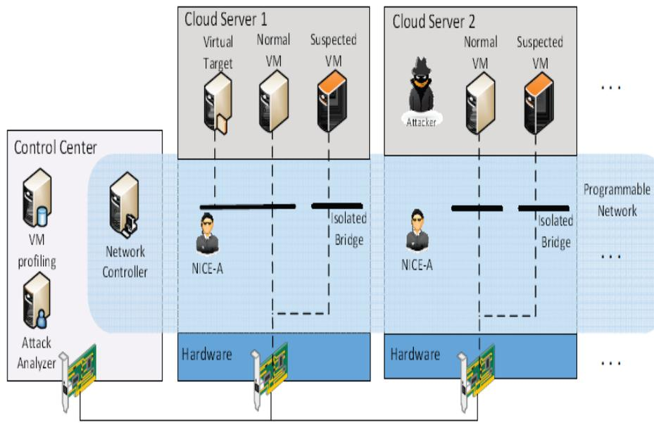
Fig.1: System Architecture within one server cloud cluster
